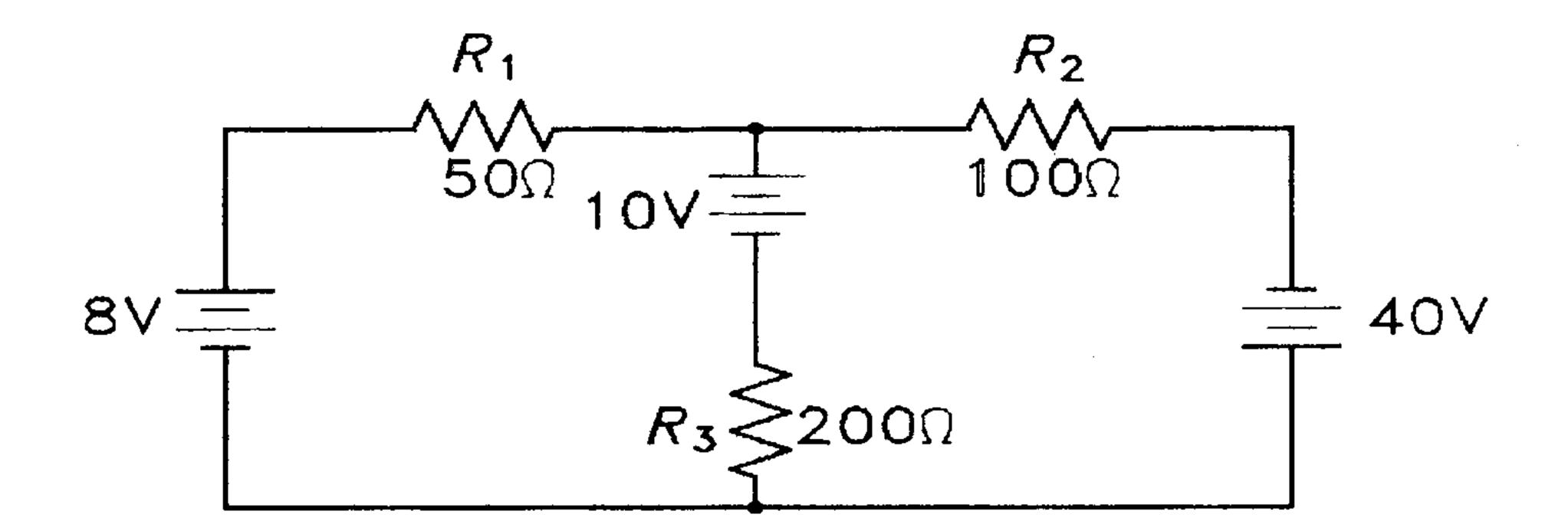
b. Determine the current drawn from the supply using start delta conversion. (5)
